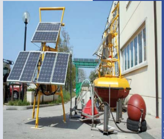
Figure 2 Monitoring buoy with solar panels for energy supply, floats and device to sample gas at the bottom of the sea.
