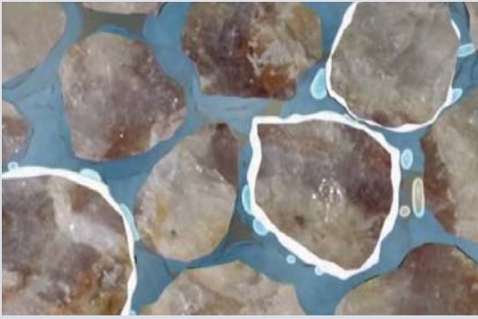
Figure 2 Dense CO 2 migrating upwards (light blue bubbles), dissolving and reacting with the grains of the rock, leading to precipitation of carbonate minerals on the grain boundaries (white).
